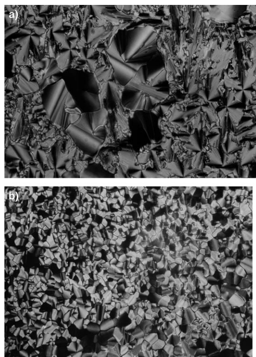
Figure 1. Optical texture (magnification 40 \times ) of the hexagonal columnar mesophase of compound: a) [Ag(L * ) 2 ][OTf] ( 3 ) as observed on cooling at 83 °C; b) [Ag(L * ) 2 ][DOS] ( 4 ) as observed on cooling at 31 °C.
